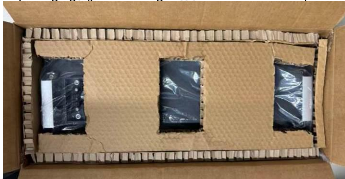
Inner packagings (protection against short circuit and displacement)
