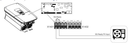
Using the **SG Ready** function is a simple and cost-effective solution to increase PV self-consumption by using a heat pump. The inverter allows a heat pump with **SG Ready** compatibility to be controlled.
