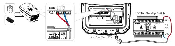
✓ The KOSTAL BackUp Switch signal cable is connected.
