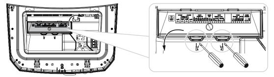
4. Insert the DC overvoltage module in the slot until it engages.
