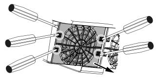
**4.** Completely remove the fan unit from the housing. To do this, disconnect the plug of the fan cable.
