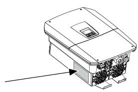
The type plate and other labels are attached to the device housing. These signs and labels must not be altered or removed.
