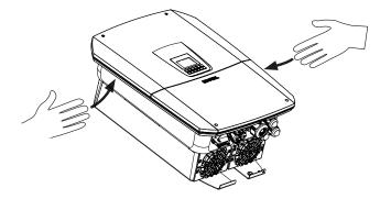
For enhanced inverter transport, use the grip strips on the left and right side of the inverter.
