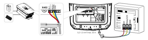
✓ The automatic backup box's signal cable is connected.
