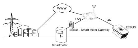
Using a smart meter gateway connected to the inverter, the energy supplier can control the inverter via the EEBus protocol to regulate the feed-in of the PV system.
