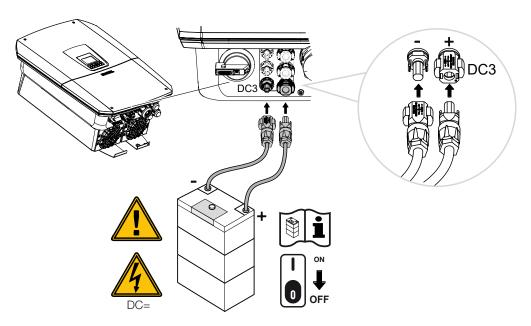
✓ The battery's DC cables are connected.
