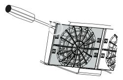
**3.** With a second screwdriver, press the fastening straps toward the centre of the fan. Pull the fan unit slightly forward.
