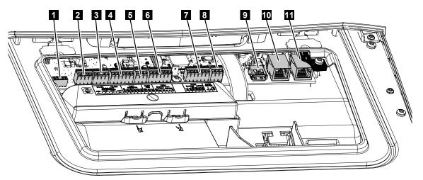
The Smart Communication Board (SCB) is the communication and interface centre. All the connections for communicating with other components can be found on the SCB.
