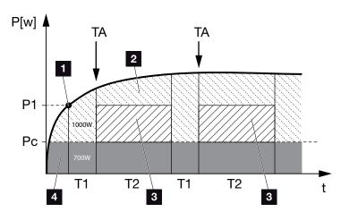
Fig. 68: Dynamic self-consumption graph (Function 1) Power limit
