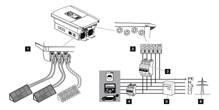
Fig. 20: Overview of electrical connections
