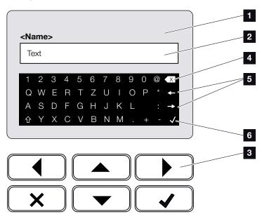
Fig. 44: Using keyboard to operate the display
