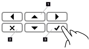
Fig. 43: Operation of the display
