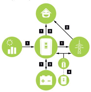
Fig. 15: Control and distribution of the energy flows
