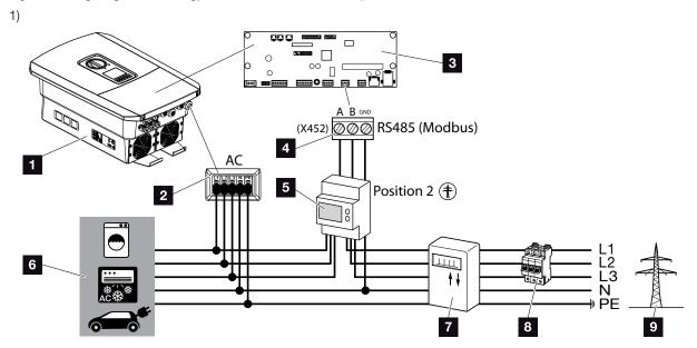
Fig. 28: Wiring diagram for energy meter - grid connection (position 2)
