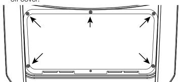
Fig. 22: Taking off terminal compartment cover
