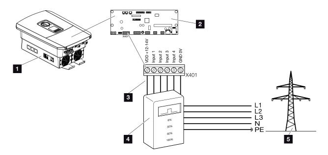
Fig. 30: Ripple control receiver
