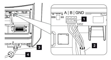
Fig. 29: Connection for digital energy meter (Modbus RTU)
