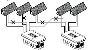
Fig. 39: Incorrect connection of PV generators
