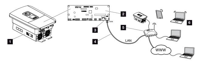
Fig. 33: Communication connection
