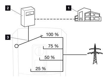
Fig. 60: External battery control via digital inputs
