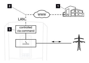
Fig. 59: External battery control via Modbus (TCP)
