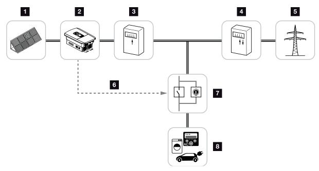
Fig. 64: Configuration of self-consumption control
