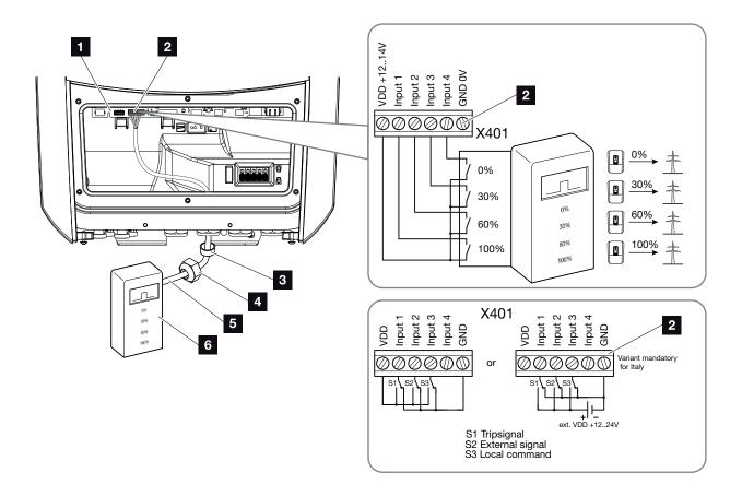
Fig. 31: Connection of ripple control receiver
