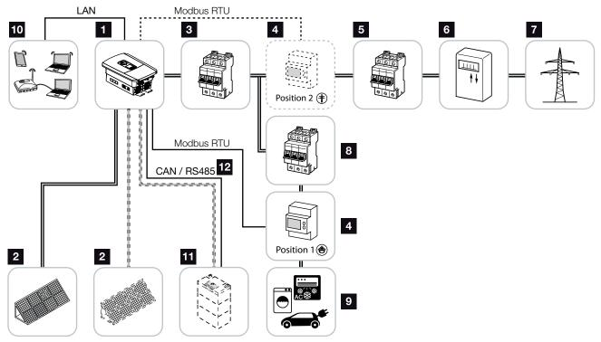
Fig. 8: Photovoltaic system with PV and battery connection
