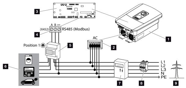
Fig. 27: Wiring diagram for energy meter - house connection (position
