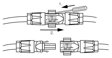
Fig. 41: Disconnecting SUNCLIX DC plug
