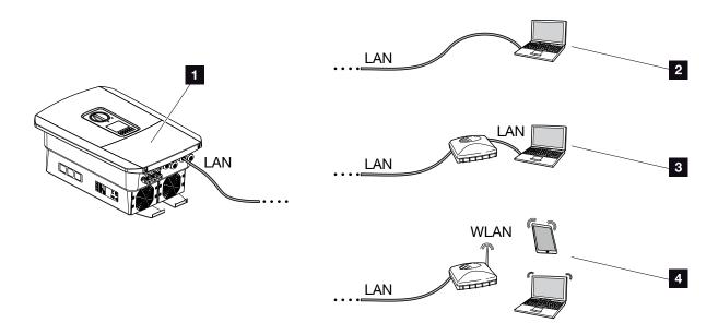
Fig. 50: Connection from computer to inverter
