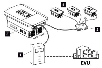
Fig. 62: Inverter with ripple control receiver
