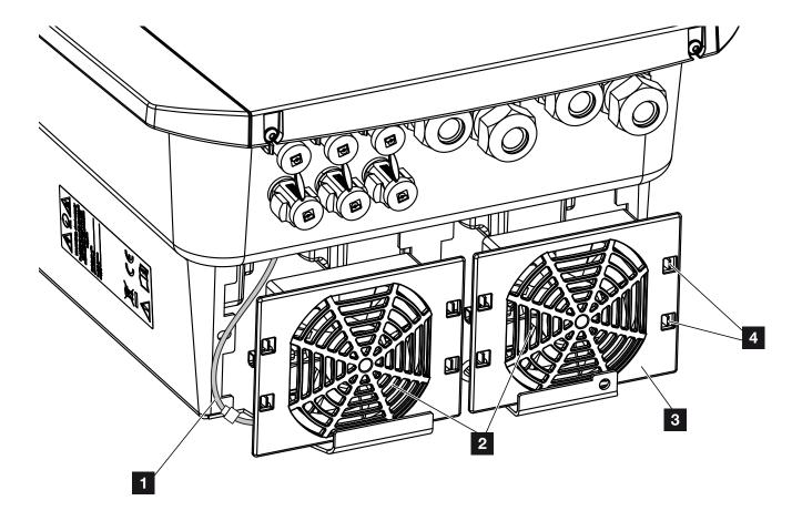
Fig. 72: Fan disassembly overview
