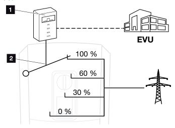
Fig. 61: Active power control with ripple control receiver
