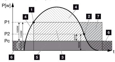
Fig. 70: Dynamic self-consumption graph (Function 2)
