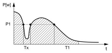
Fig. 71: Brief delay in drop in output/fault
