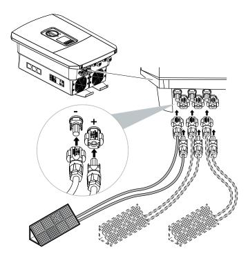
Fig. 40: Overview of DC connections
