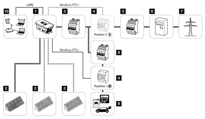
Fig. 7: Photovoltaic system with 3 PV inputs
