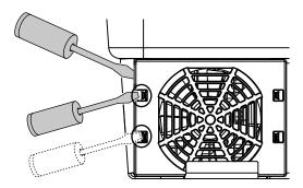
Fig. 74: Loosen fastening straps
