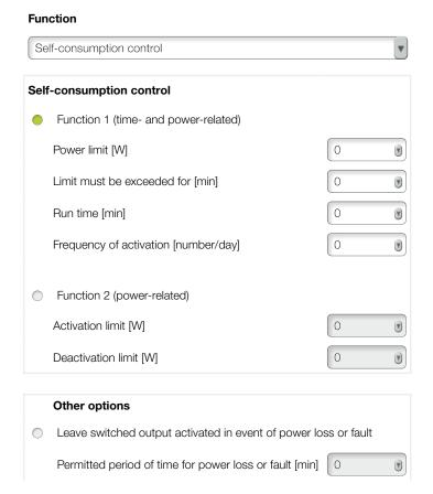
Fig. 66: Self-consumption control functions for Webserver
