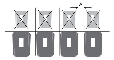
Fig. 19: Wall mounting of several inverters
