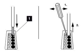
Fig. 24: Spring-loaded terminal strip
