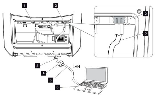
Fig. 34: Connecting inverter and computer with an Ethernet cable
