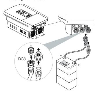
Fig. 38: Overview of battery DC connection
