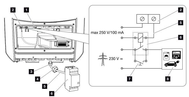
Fig. 65: Electrical connection for self-consumption control
