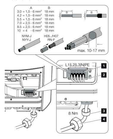
Fig. 23: Connecting mains cable to the inverter
