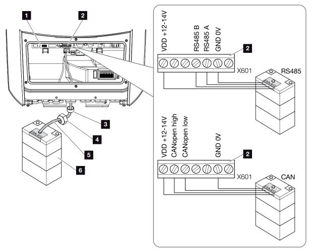
Fig. 36: Battery communication connection via RS485 or CAN
