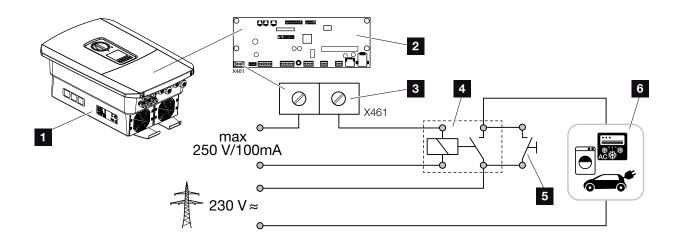
Fig. 32: Connection for self-consumption control
