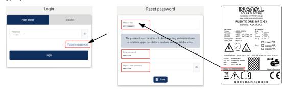
To log in as an *installer*, you need the master key from the inverter's type plate and your service code, which can be requested from our service team.
