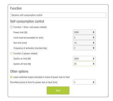
Activate the dynamic self-consumption control function in the PLENTICORE plus Webserver by going to **Service menu > Switched output**.
