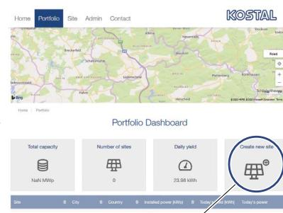
Create a new plant and add the new device to the plant /
